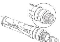
(3) Refit the hose and tighten the ball nut on to the second stageusing 11/16" spanner to hold the heat exchanger. Tighten if possible, using an 11/16" crowfoot torque wrench to 5Nm.
