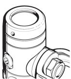
This helps to prevent ice from forming inside the ambient chamber, and also extends the life of the first stage internal diaphragm. It is important to remember, however, that this environmental protection will not completely prevent the second stage from icing or freezing.
