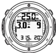
UPWARD POINTING ARROW, BLINKING ASC TIME AND AN ALARM TELL YOU TO ASCEND. MINIMUM TOTAL ASCENT TIME INCLUDING SAFETY STOP IS 9 MINUTES. CEILING IS AT 3 M.
