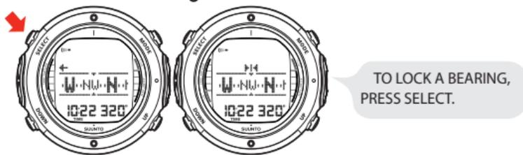
The Suunto D6i also provides help for navigating square and triangular patterns, as well as navigating a return heading. This is made possible by following graphical symbols in the center of the compass display:
