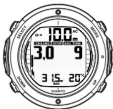
UPWARD POINTING ARROW HAS DISAPPEARED AND ASC TIME LABEL HAS STOPPED BLINKING, MEANING YOU ARE IN THE DECOMPRESSION RANGE.
