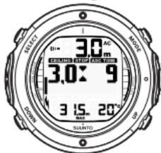
TWO ARROWS POINT AT EACH OTHER "HOUR GLASS" YOU ARE IN THE OPTIMUM CEILING ZONE AT 3 M AND YOUR MINIMUM ASCENT TIME IS 9 MINUTES.
