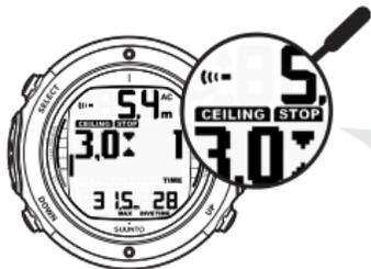
WHEN CEILING AND STOP ARE DISPLAYED, MAKE A ONE MINUTE MANDATORY SAFETY STOP IN THE DEPTH ZONE BETWEEN 6 M AND 3 M.
