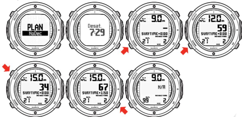
WHEN ENTERING THE PLAN MODE THE DISPLAY FIRST BRIEFLY SHOWS THE REMAINING DESATURATION TIME BEFORE GOING INTO PLAN MODE. USE UP AND DOWN BUTTONS TO SCROLL NO-DECOMPRESSION LIMITS AT DIFFERENT DEPTHS. YOU CAN ALSO ADJUST YOUR SURFACE INTERVAL TIME TO YOUR PLAN. NO-DECOMPRESSION LIMITS LONGER THAN 99 MINUTES ARE DISPLAYED AS “—”.
