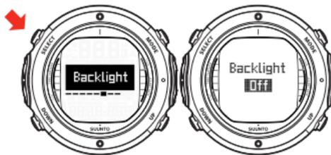
ADJUST WITH UP AND DOWN BUTTONS. ACCEPT WITH SELECT BUTTON.
