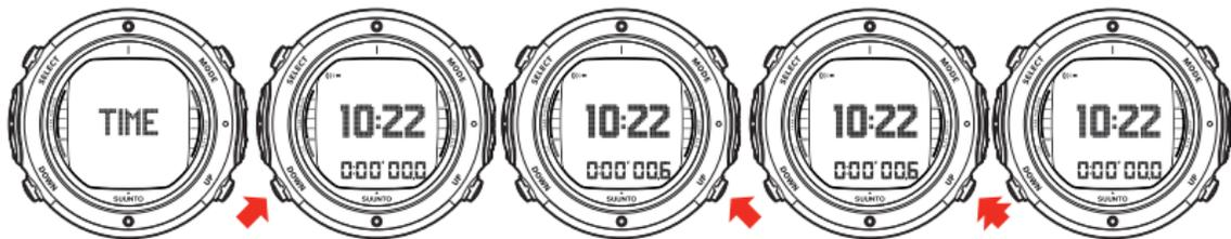
USE DOWN BUTTON TO START STOPWATCH AND TAKE A SPLIT TIME. THE UP BUTTON STOPS THE STOPWATCH AND LONG PRESSING IT RESETS IT.
