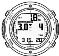
WHEN CEILING AND STOP ARE DISPLAYED WITH DOWNWARD POINTING ARROW, IMMEDIATELY (WITHIN 3 MINUTES) DESCEND TO OR BELOW CEILING.
