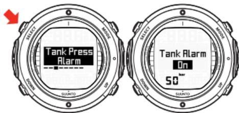
TANK PRESSURE HAS DROPPED BELOW 50 BAR AND THE REMAINING AIR TIME IS 4 MINUTES. THE DISPLAY BLINKS AND THERE IS AN AUDIBLE ALARM.
