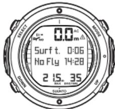
IT IS 6 MINUTES SINCE YOU SURFACED FROM A 35-MINUTE DIVE. THE MAXIMUM DEPTH WAS 21.5 M. THE PRESENT DEPTH IS 0.0 M. THE AIRPLANE SYMBOL AND NO-FLY VALUE INDICATE THAT YOU SHOULD NOT FLY FOR 14 HOURS, 28 MINUTES. THE DIVER ATTENTION SYMBOL INDICATES THAT YOU SHOULD PROLONG YOUR SURFACE INTERVAL TIME.
