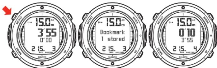
BY PRESSING THE SELECT BUTTON DURING A DIVE, A BOOKMARK IS WRITTEN IN THE PROFILE MEMORY, THE DIVE TIMER IS RESET, AND THE PREVIOUSLY-TIMED INTERVAL IS DISPLAYED BELOW.
