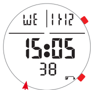
LOW BATTERY (YOU SHOULD CHANGE THE BATTERY SOON)
