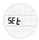
Smart Air's **SEt** menu allows you to change settings. Once inside this menu, press the **UP** or **DOWN** button to scroll between two submenus: **SEt dIVE**, where you can set parameters pertaining to the dive, and **SEt tIME**, where you can set parameters pertaining to time and date.
