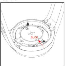
f) Position the new o-ring from the kit in the groove around the battery, ensuring that it sits towards the outer edge of the groove.
