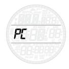
This submenu allows you to download your dive data to a PC or Mac. Press the **ENTER** button and the display will show **PC ready**, symbolizing that Smart Air is ready to communicate.
