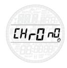
Press and hold the **UP** button to enter this menu. The middle row now features a stopwatch while the time of day has moved to the bottom row. Press the **UP** button to start and stop the time, then press the **DOWN** button to reset the time to zero. Press and hold the **DOWN** button to exit from the stopwatch function (this stops and resets the stopwatch if it was running or stopped at a non-zero value upon exiting).
