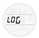
Smart Air can record the profiles of approximately 95 hours of diving, at a sampling rate of 5 seconds. The information can be transferred using the optional USB clip to PC via the Dive Organizer software or to a Mac via the Divers' Diary software. In addition, Smart Air can show most of the information directly on the display.
