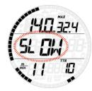
If the ascent rate exceeds 12m/min / 40ft/min at a depth below 12m / 40ft, # blinks as well. If a speed in excess of 12m/min / 40ft/min is maintained for two thirds or more of the depth at which the alarm was first triggered, Smart
