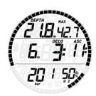
If you press the **DOWN** button while G2 is blinking, the next available gas in the list will be displayed instead. This will be G1 if only two gases are set or if you are deeper than the MOD of G3, or G3 if you have set three gases and are shallower than the MOD of G3.
