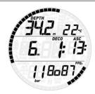
In case of an ascent, the **speed** in m/min or ft/min is displayed in the bottom left corner.
