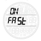
A fast (uncontrolled) ascent is defined as one in which a speed of 12 m/min / 40ft/min or higher was maintained over more than two thirds of the way up. This applies to dives deeper than 12m/40ft only. In such an event, due to the potential of harmful bubble formation, Smart Air locks the computer for 24 hours in order to discourage you from diving again. In this menu, you have the option to disable the locking up of the computer in the event of an uncontrolled ascent.
