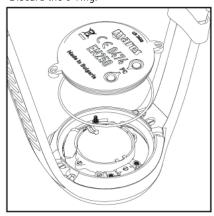
d) Remove the battery by prying it loose with a small flat-head screwdriver.
