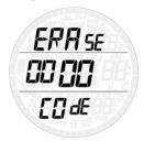
Smart Air allows you to reset the desaturation in the computer. Any tissue saturation information from a recent dive will be reset to zero and the computer treats the next dive as a non-repetitive dive. This is useful when the computer is loaned to another diver who has not dived in the last 24 hours.
