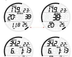
By pressing the **UP** button, you can modify the information displayed in the upper row. At each button press, the screen cycles through temperature, max depth, average depth, MOD (nitrox only), deep stop (if activated and if calculated to be present), and an empty field.
