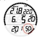
Press and hold the **DOWN** button to confirm the switch to G2: the set oxygen concentration will be displayed steadily in the lower right corner of the screen, and within 20 seconds the ascent time is updated to reflect the higher oxygen concentration in the breathing gas.
