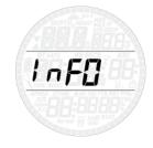
This submenu provides information about the hardware and software of your Smart Air and about the status of the battery: **OK** means the battery is good, **LO** means the battery is weak but you can still do a few more dives, and **KO** means the battery is very low and Smart Air won't function as a dive computer.
