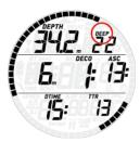
Upon reaching the optimum range for carrying out a deep stop (+/- 1m /3ft of the displayed depth), the deep stop itself will be shown in the top right corner with the label **DEEP** blinking, and a countdown timer appears to indicate the progress of the stop. Deep stops can be deactivated in a dedicated settings menu.
