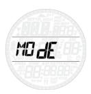
Here you can define the type of gas you will be breathing during the dive (air or enriched air nitrox, including multigas). You can also set Smart Air to bottom timer (BT), in which case Smart Air will show only time, depth, tank pressure and temperature: it will not carry out any decompression calculation and it will not show any warnings and alarms. You can set Smart Air also to APNEA, which in essence is a bottom timer with special features dedicated to apneists.
