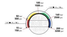
The tank pressure can be displayed also numerically by pressing and holding the **DOWN** button. In NO DECO this moves the dive time to the left of the center row while the no deco time is shifted to the right. In DECO this replaces the dive time with the tank pressure. By pressing and holding the **DOWN** button again, the displays revert back to the previous lay-out.
