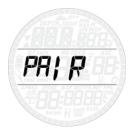
The display will show **G1** in the lower right corner and the word **PAIR** in the middle. The lower left corner shows the letters **nP** (Not Paired) or **P** (Paired) to indicate the current status of that channel. Use the **UP** and **DOWN** buttons in case you are trying to pair channel **G2** or **G3**.
