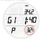
Once inside this menu, press the **UP** or **DOWN** button to change the  $0_2$ % and observe how this affects the maximum operating depth (MOD). Then press and hold the **UP** button to move on to the pp $0_2$ max and use the **UP** or **DOWN** button to change the value, again noticing how this affects the MOD. Press and hold the **UP** button again to save the setting.
