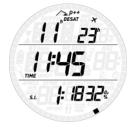
The post-dive display is the default display for as long as either the no-fly or the desaturation is greater than 0 minutes. By pressing the  $\bf DOWN$  button you can go to all other screens but Smart Air will revert automatically to the post-dive display after an 8-second time out. For as long as there is desaturation, Smart Air also features a condensed log of the last dive: maximum and average depth in the top row, dive time and set 0.2% in the bottom row.
