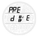
Press and hold the **UP** button to enter this menu and put Smart Air into the ready-to-dive mode.
