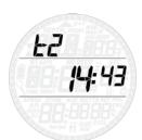
Smart Air features a "sleep" mode: in case you don't wear it other than on a dive trip, you can put Smart Air in sleep mode to reduce battery consumption. This turns off the display while
