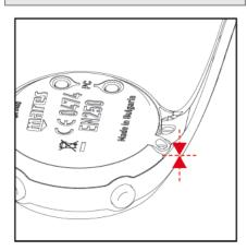
h) Keep the cover pressed onto the watch case while hand tightening the two screws. Don't use excessive force while tightening. Ideal torque is 12 N cm / 17 oz-in.
