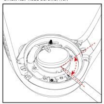
e) Replace the battery with the new one from the kit. The battery should click in place. Make sure to respect the correct polarity of the battery: the "+" has to be facing outwards.
