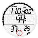
In this case, if the diver attempts a repetitive dive after surfacing, Smart Air will only function as a depth gauge and timer (bottom timer mode), and will display  $\widehat{I}$  on the screen throughout the dive.
