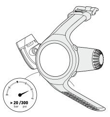
Press ENTER and wait until OK appears on the display, in which case you have successfully established a connection. If OK does not appear on the display you need to repeat the operation, but you must turn off the valve and depressurize the first stage completely, then wait 20 seconds before attempting again.
