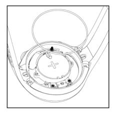
g) Position the cover onto the watch case and press it down evenly. Ensure that in the area of the screws the cover touches the watch case.
