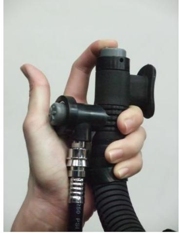
\* Due to technical wing's inherent design, sometimes gas may get trapped inside your the wing. Therefore when venting gas from the air cell while diving with the power inflator, make sure the inflator elbow is at the highest point (i.e. above the rest of the wing) and hold the power inflator as high as you possible can before depressing the button.
