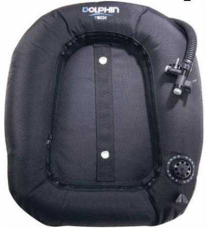
For JT-30 single tank and JT-50 twin tank (right) air cells, each has a single inner bladder and comes with a single 16" inflator with standard technical elbow connection and an over-pressure exhaust valve to the front lower left side (when wearing). They have 1 pair of grommets at industry standard 11" apart.
