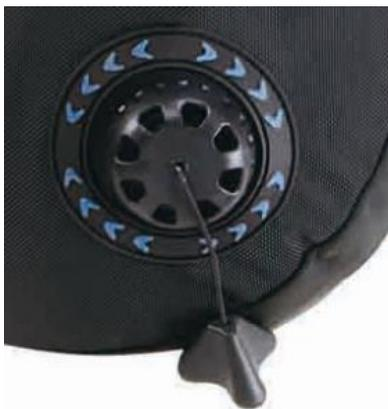
Each air cell discussed previously is equipped at least 1 rapid exhaust valve which automatically releases excess gas when the pressure inside the bladder is 0.17kg/cm<sup>2</sup> (2.4psi) greater than the ambience to protect the bladder from bursting.
