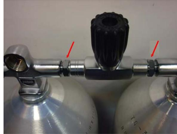
2) Make sure these lock nuts are shifted all the way towards the centre isolator valve to allow room for adjustment later. You will need a (adjustable) spanner with 22mm jaw opening. Please note the right valve's thread (pictured left) is left-handed, turn clockwise to loosen.
