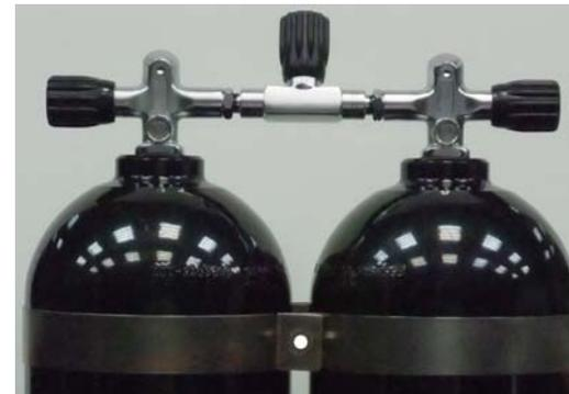
4) Place the other band at or just below where the cylinder dome curve ends.
